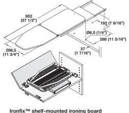
Ironfix<sup>™</sup> shelf-mounted ironing board Height: 130 mm (5 1/8") Width: 520 mm(20 1/2") Depth: 350 mm (13 3/4") Extended board length is 952 mm (37 1/2") Material: steel, epoxy-coated Cover: natural white cotton with gray stripes, foam backed
